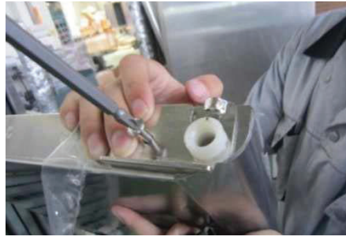
G. Assemble stopper plate in original positions.
