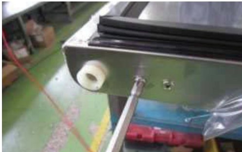
F. Disassemble stopper plate, then tight screws.
