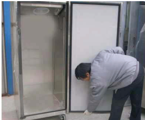
B. Lift the door, then remove it.
