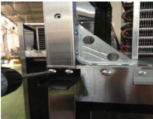
C-1. Disassemble the top hinge (left).
