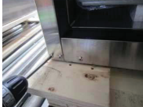
C-2. Disassemble bottom hinge (left).
