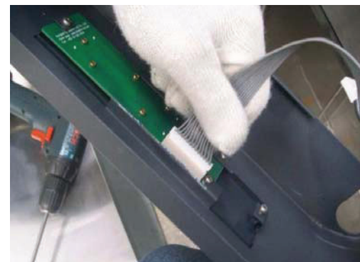
E. Pull out the harness of the display PCB and the harness of the door s/w located on back of top grille (B).
